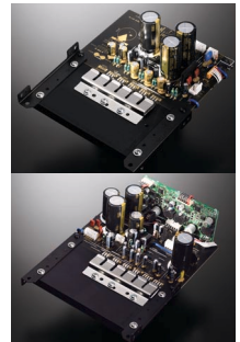
Digital power circuit board (top) and analog power board (bottom)
